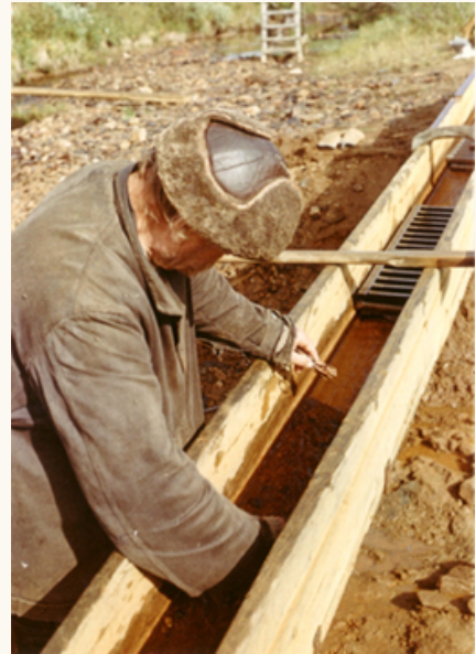
A miner uses a sluice to wash gold from sediment in 1960. Modern placer mining uses larger, mechanized sluices and gravity systems to do the same work.
