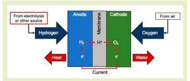
In a hydrogen fuel cell, hydrogen reacts with oxygen producing water and heat.
