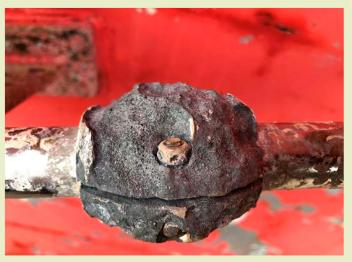
This worn galvanic anode (also known as a sacrificial anode) protects the steel of a yacht's propeller shaft. Material is lost from the anode rather than the metal of the shaft, protecting the shaft from rusting.
