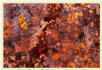
Layers of rust flake off of exposed iron metal because the hydrous ferric oxide molecules are larger than the iron atoms they replace, so they can't fit back into the space left by dissolution of the iron atoms.
