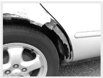
The fender of this car has rusted through, probably because of salting to melt ice on roads.
