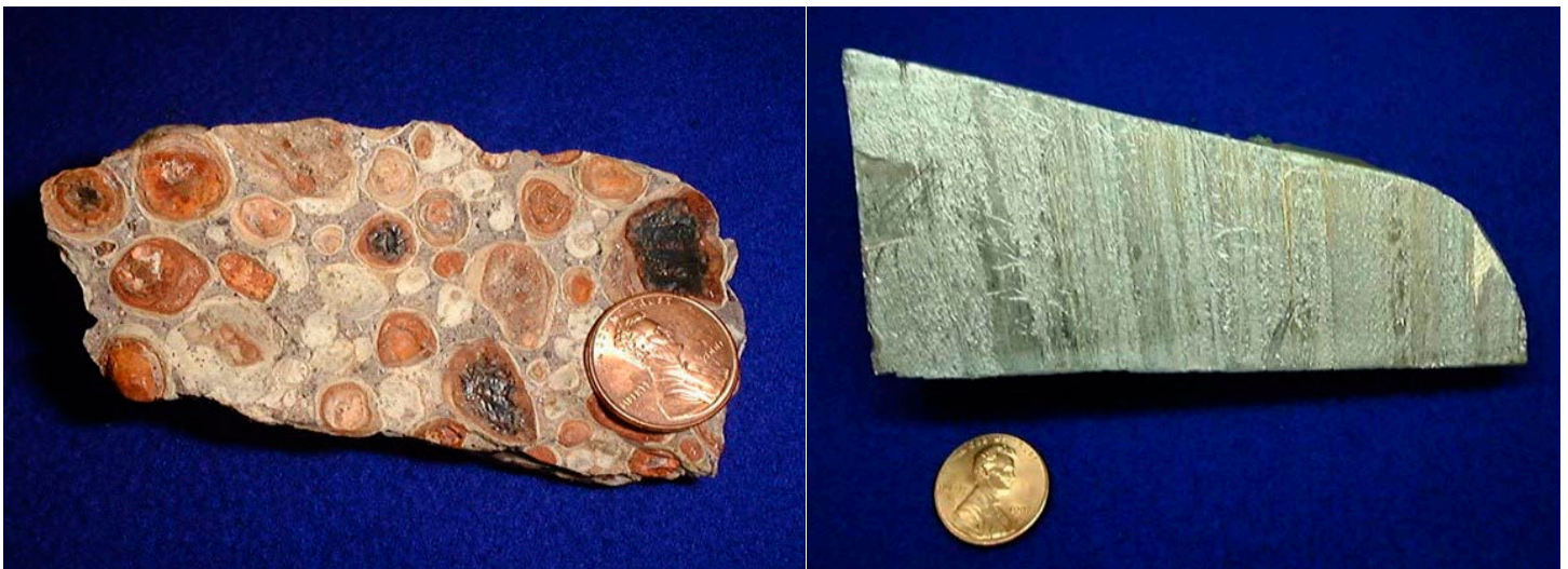
Bauxite from Les Baux-de-Provence, France, and a piece of aluminum metal, with U.S. pennies for comparison. Bauxite forms as a rind on the rock fragments in this conglomerate.
