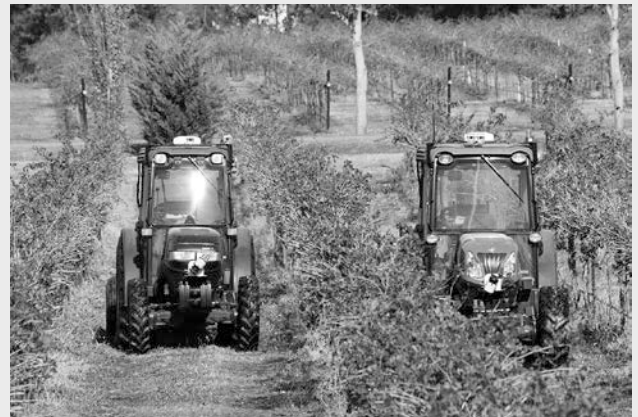
Two autonomous compact tractors performing spraying functions in a Texas vineyard. Each driverless tractor is controlled from a single command station.
