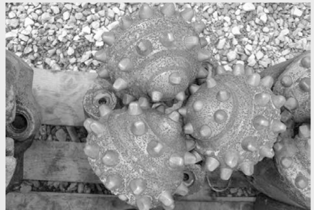
A tricone roller cone drillbit assembly showing the protruding tungsten carbide buttons inset into the rollers.
