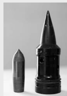
Armor-piercing discarding-sabot tracer round for 17-pounder gun (WW2), with its tungsten carbide core from Canadian Arsenals. Kinetic bombardment uses superdense material like tungsten carbide to breach armor instead of explosives.
