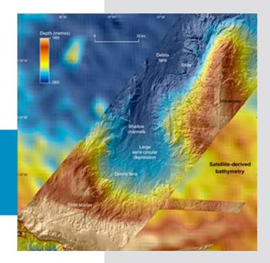
Differences in resolution between multibeam and satellite-derived bathymetry data for a part of the Indian Ocean floor are striking. This detailed survey was completed during the search for Malaysian Airlines Flight 370, which disappeared March 8, 2014.
