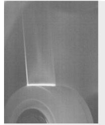
Sticky tape emits light as it unpeels in the presence of air, but in a vacuum, it emits X-rays in the absence of nitrogen.
