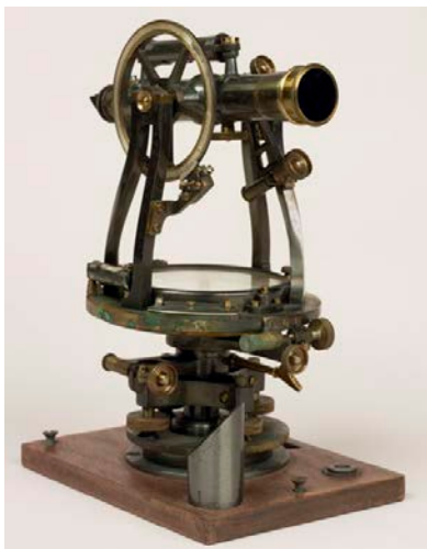
A surveying theodolite from the early 20th century.
