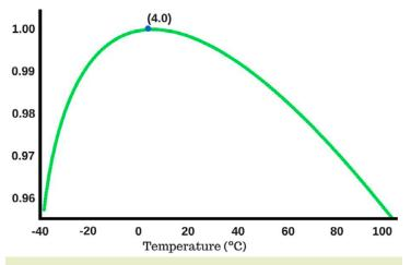
This graph shows the density of H<sub>2</sub>O versus temperature. Water molecules are polar, and they repel each other like little magnets as they crystallize into ice. This makes water's solid form less dense than its liquid form. Most other solids are denser than their liquid form.
