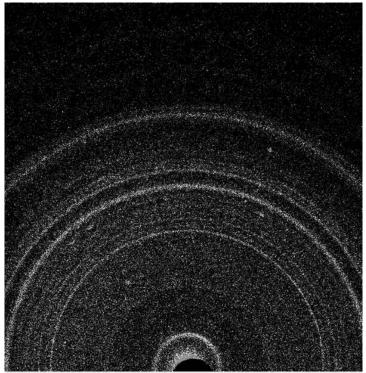
This graphic shows results of the first analysis of Martian soil by the Chemistry and Mineralogy (CheMin) experiment on NASA's Curiosity rover in October 2012. Each dot in this diffraction pattern was formed by the constructive interference of scattered X-rays passing through a crystal. This soil sample, taken from a wind-blown deposit within Gale Crater, is similar to volcanic soils in Hawaii.
