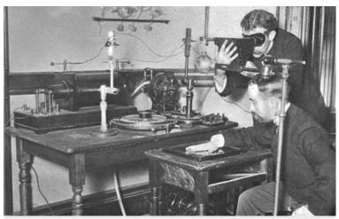
A photo from 1896 of experimenters taking an X-ray with an early Crookes tube. The Crookes X-ray tube, which looks like a lightbulb, is visible suspended near the center of the photo. The standing man is examining the bones of his hand with a fluoroscope screen, while the sitting man is taking a radiograph of his own hand with a photographic plate. Neither of them are taking precautions against radiation exposure; its hazards were not known at the time.
