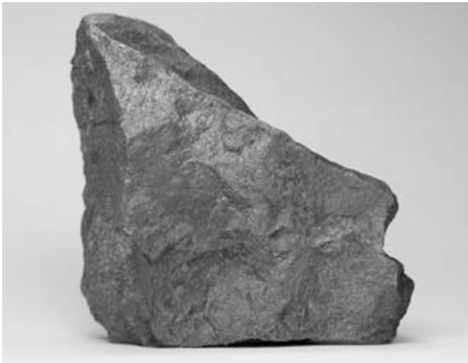
A sample of magmatic nickel sulfide ore from the Sudbury Igneous Complex. This is a specimen of pentlandite in pyrrhotite approximately 4 inches across.
