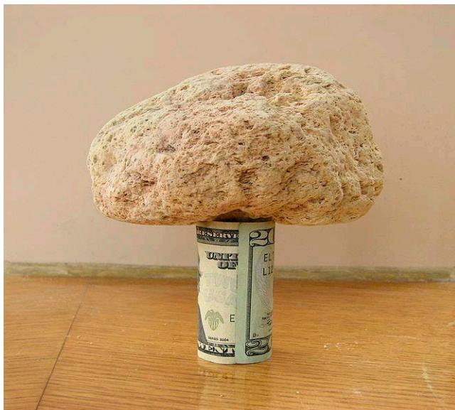
A 6-inch (15-centimeter)-wide piece of pumice rests on a rolled-up US \$20 bill, demonstrating its extremely low density.
