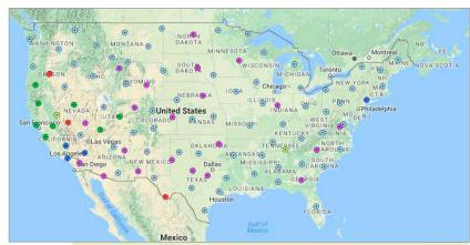
The USGS Reference Station Network forms the backbone of the lower 48 United States seismic array.
